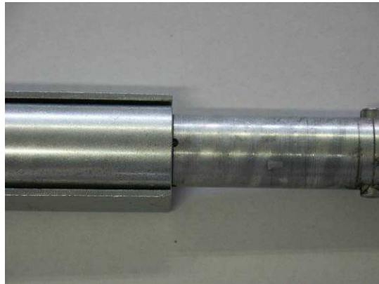
Figure 7: Middle of the pilot hole aligned with the edge of the guide bushing
